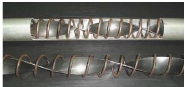
Fig. 2 Riser tube with wire coil and twisted tape
