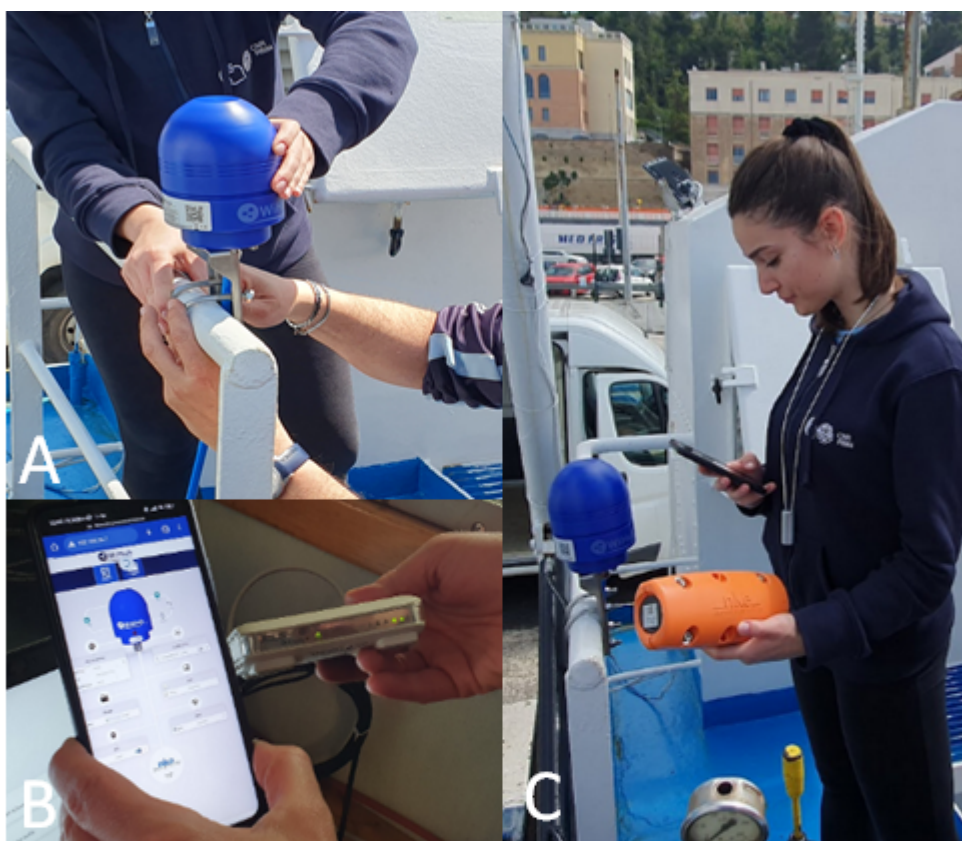
Figure 33: A) WiHub installation operations on board R/V Dallaporta; B) WiHub web interface; C) Setting of the sensor through the web application.
