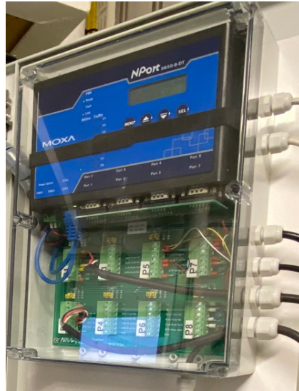
Figure 73: FerryBox serial-to-Ethernet interface junction box with Moxa NPort and serial device connection board.
