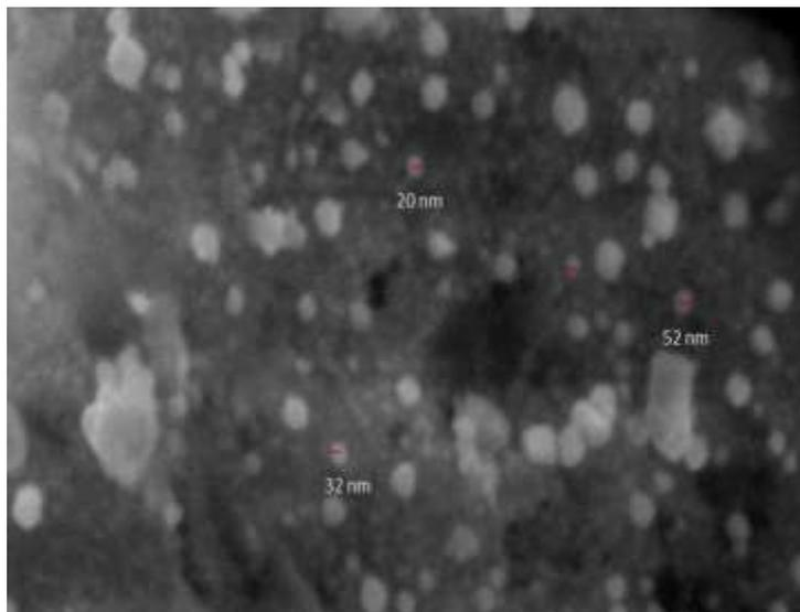
**Figure 4: SEM Image of Silver Nanoparticles**
