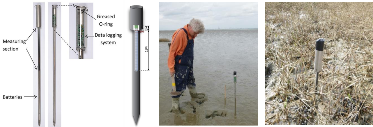
Figure 2.1 Left: front side and back side and an enlargement of the logging section of the SED-sensor (Hu et al., 2015). The light sensitive cells are located in the measuring section, and the head. Middle: a SED-sensor on the mudflat. Right: a SED-sensor in the marsh, Paulinapolder, the Netherlands, April 2014.
