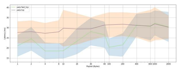
Figure 36. UC9 - Latency vs payload for the Protocol test (from B to A endpoint).
