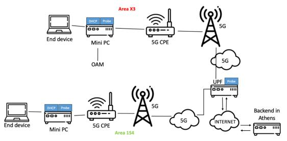
Figure 26. UC6 – Testbed Architecture.
