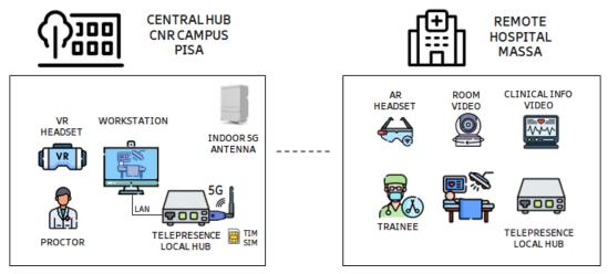
Figure 15. UC7 - Remote Proctoring – Architecture and main components.
