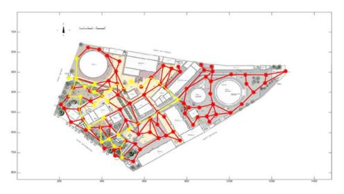
Figure 14. UC6 – Optimal route calculation for the Evacuation.
