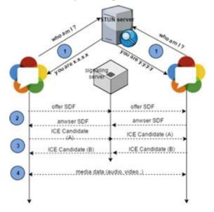
Figure 19. UC7 - Connection Negotiation and data flow.
