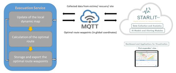
Figure 3. UC6 - High-level Evacuation Service architecture and link to the STARLIT++ platform.
