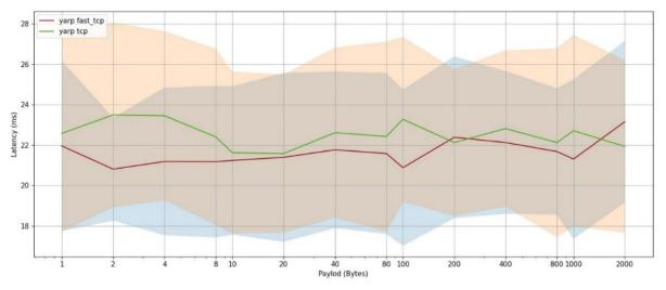
Figure 35. UC9 - Latency vs payload for the Protocol test (from A to B endpoint).
