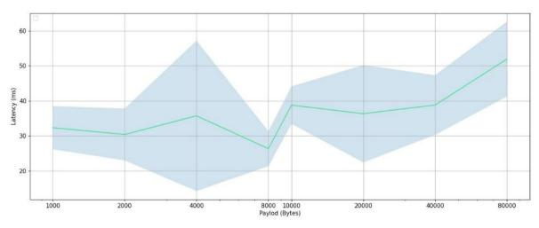
Figure 38. UC9 - Latency vs payload for the Payload test (from B to A endpoint).
