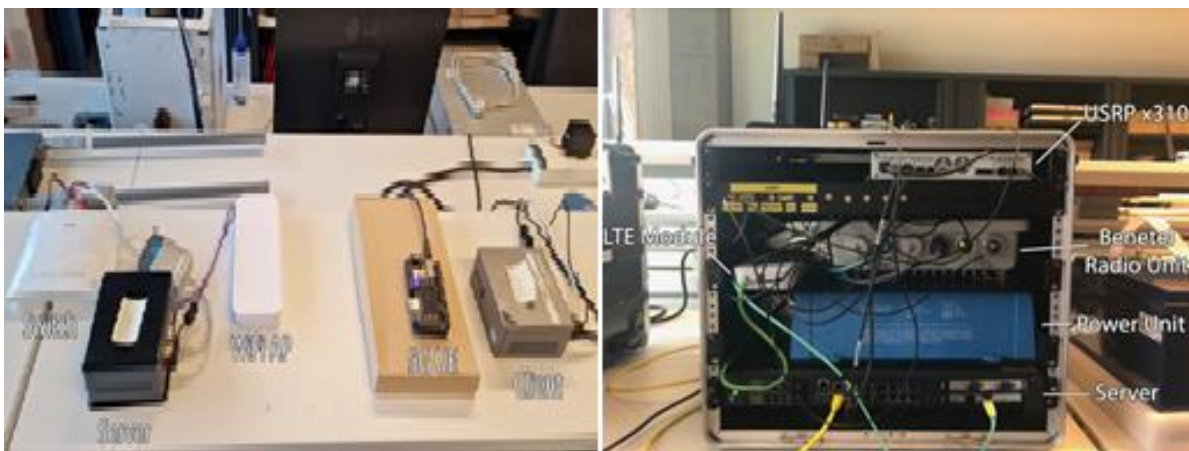
Figure 25. IMEC-Ghent 5G testbed setup.
