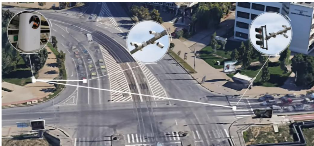
Figure 22. UC4 Podu Ros intersection surveillance cameras placement.
