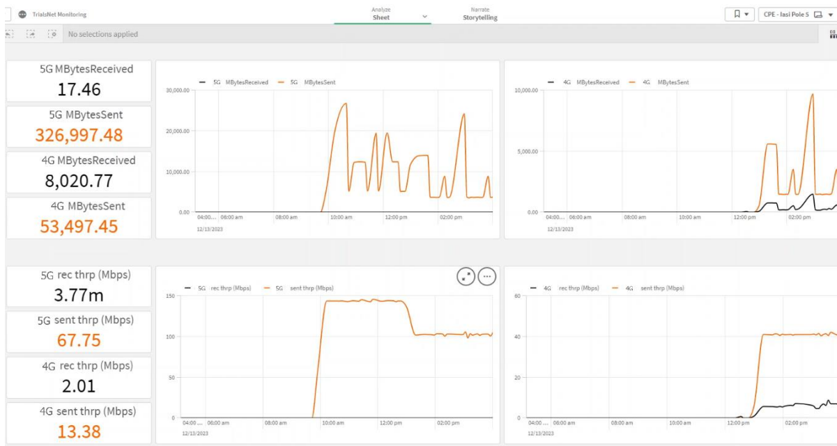
Figure 48. UC1 CPEs integration in ORO’s monitoring platform - data throughput metrics.
