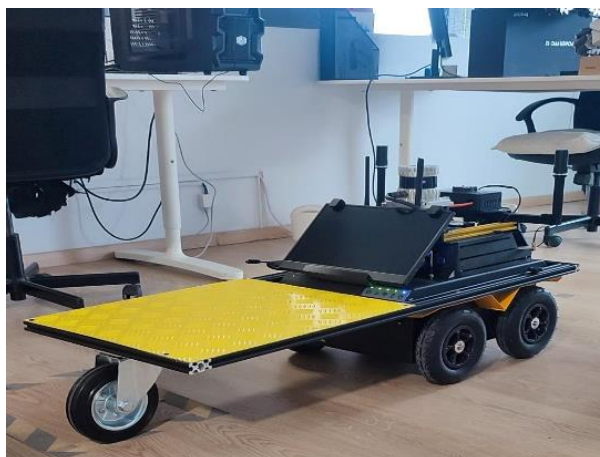
Figure 71. The Jackal robot adapted for the Autonomous APRON use case.
