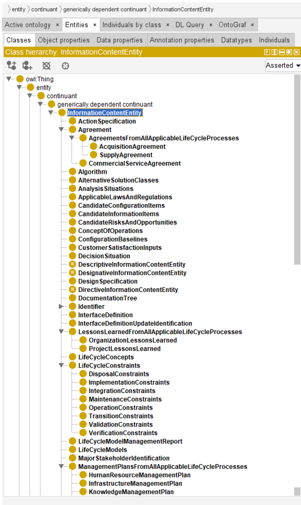
Figure 59 Taxonomy of information content entities participated in system life cycle processes (excerpt)
