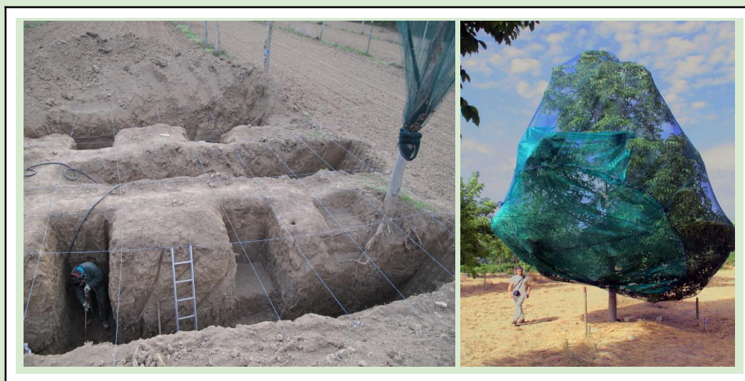
Figure 1 Measurements of C fluxes in agroforestry systems required estimating the full leaf biomass by wrapping the trees in nets (Restinclières experimental Estate, France) or measuring fine root turn-over by excavation or minirhizotrons (Photos Christian Dupraz).
