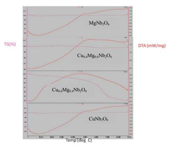
Fig. 5 TG-DTA analysis of Cu<sub>x</sub>Mg<sub>1-x</sub>Nb<sub>2</sub>O<sub>6</sub>, (x=0,0.4,0.6,1)
