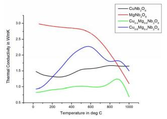
Fig. 2 Thermal conductivity over temperature of  $Cu_xMg_{1-x}Nb_2O_6$ , (x=0,0.4,0.6,1)
