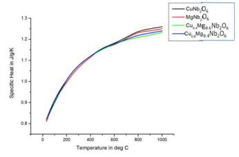
Fig. 3 Specific heat over temperature of  $Cu_xMg_{1-x}Nb_2O_6$ , (x=0,0.4,0.6,1)
