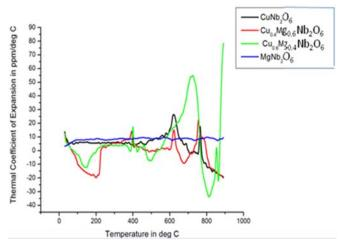
Fig. 4 Thermal coefficient of expansion over temperature of  $Cu_xMg_1$  $_xNb_2O_6$ , (x=0,0.4,0.6,1)
