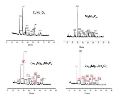
Fig. 1 XRD patterns of  $Cu_xMg_{1-x}Nb_2O_6$ , (x=0,0.4,0.6,1)
