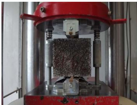
Fig. 3 Splitting tensile test
