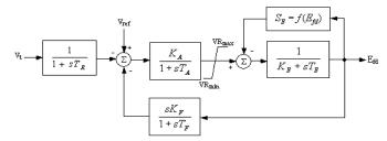
Fig. 9 Exciter block diagram
