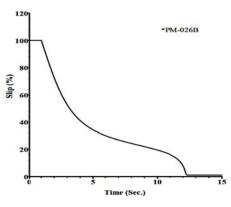
Fig 5 Motor slip during motor starting
