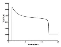
Fig. 3 Motor starting current variation with time
