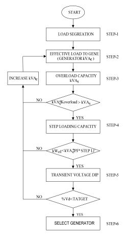
Fig. 2 Flow chart for generator sizing
