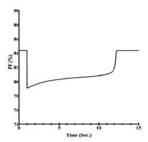
Fig. 8 Generator power factor variation during motor starting
