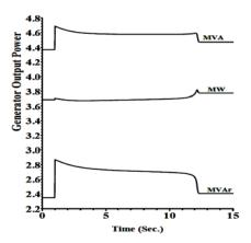
Fig. 7 Generator output power variation during motor starting
