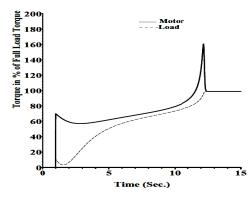
Fig. 6 Motor and Load torques during motor starting
