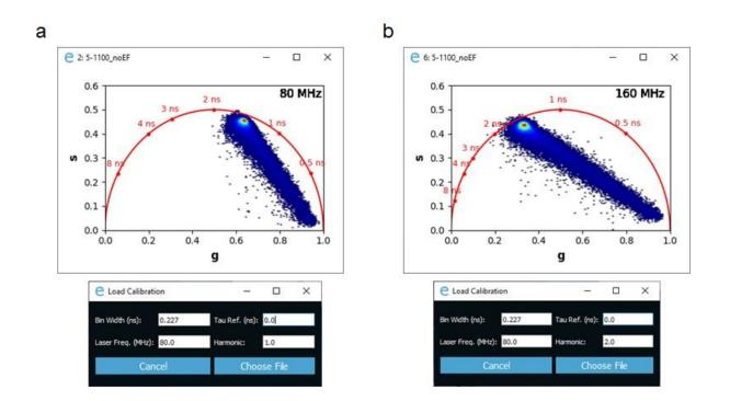
*Figure S5:* Calibration of FLIM image (ZF-1100\_noEF.tiff) using the SHG at 0 ns lifetime (starch SHG-IRF.tiff) as a calibration. Phasor transformation and plot are calculated at the first (A) and second (B) harmonic of the laser repetition rate.
