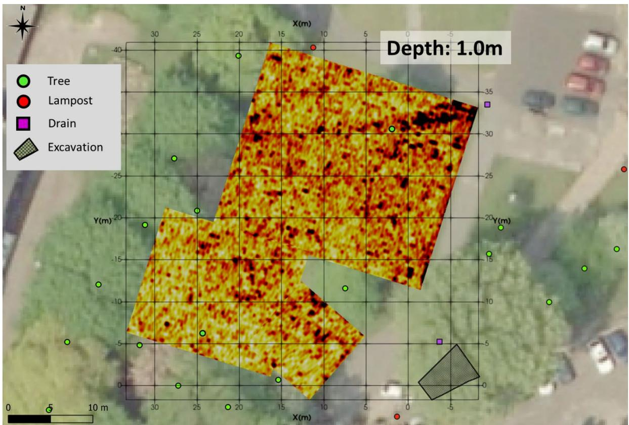
Figure 39: Horizontal slice at 1.0m from 250MHz data.
