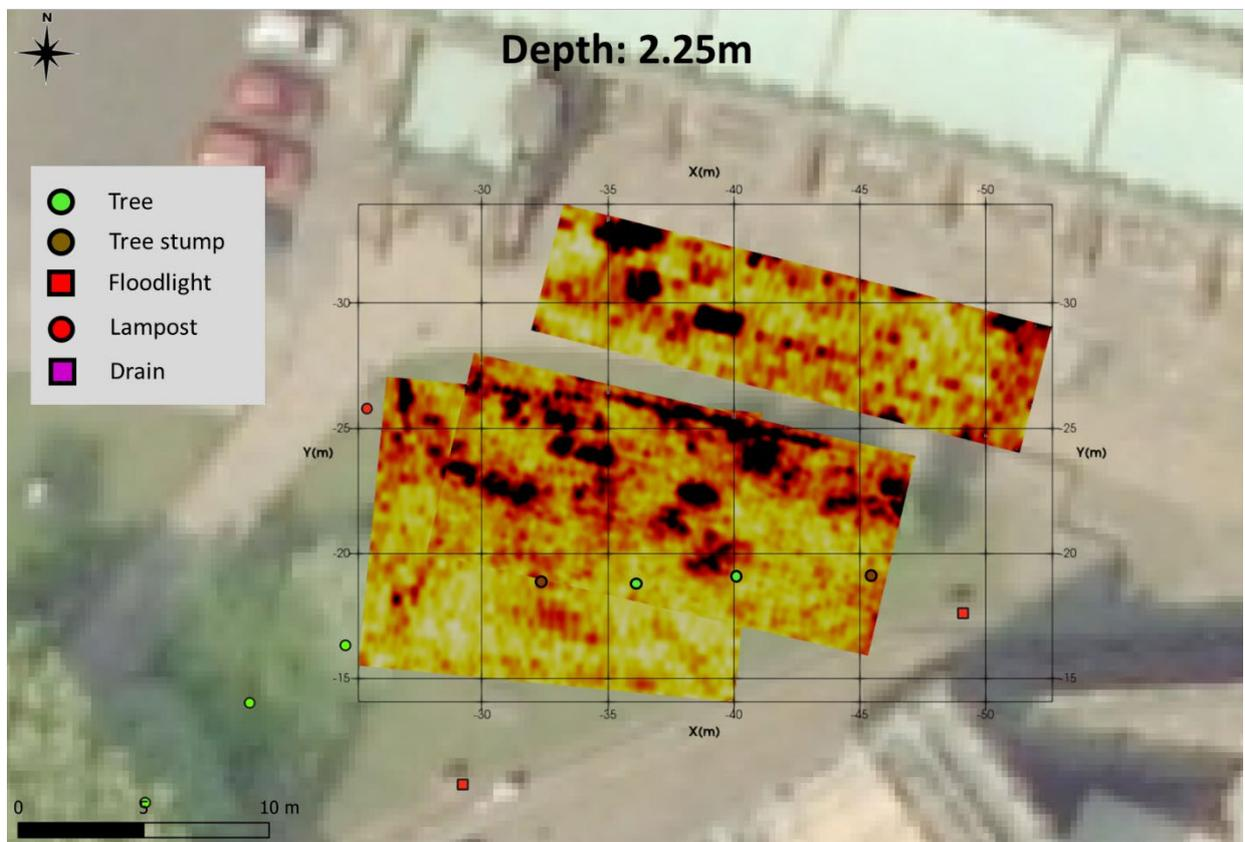
Figure 31: Horizontal slice of 250MHz data from Plots I, Q and R (depth: 2.25m).
