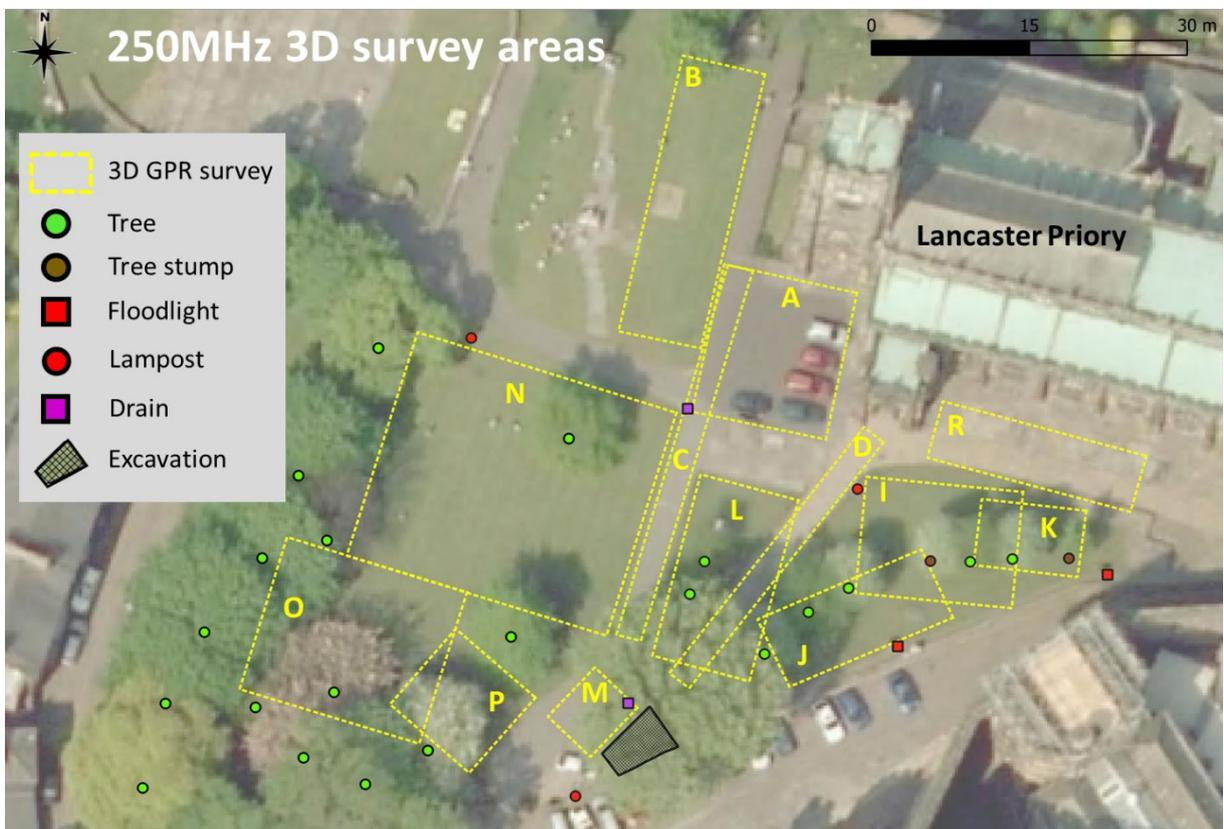
Figure 4: Coverage of 250MHz 3D surveys. An additional plot (plot Q) was also surveyed with 250MHz antenna, covering parts of plots I and K (see Table A1).
