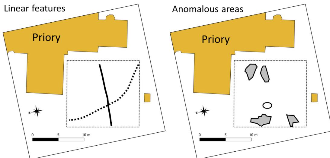
Figure 16: Summary of Plot A features. Left hand image shows linear features. Right hand image shows anomalous zones (grey filled indicate potentially electrically conductive shallow subsoil; white filled symbol shows area with potential subsoil deformation).
