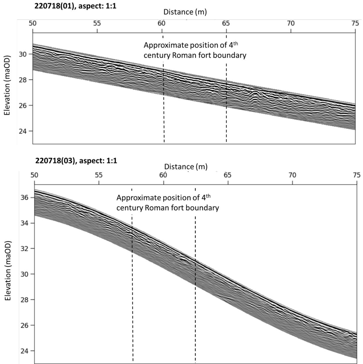
Figure 50: Sub-section of selected 250MHz surveys in the west churchyard. Refer to Figure 46 for position.
