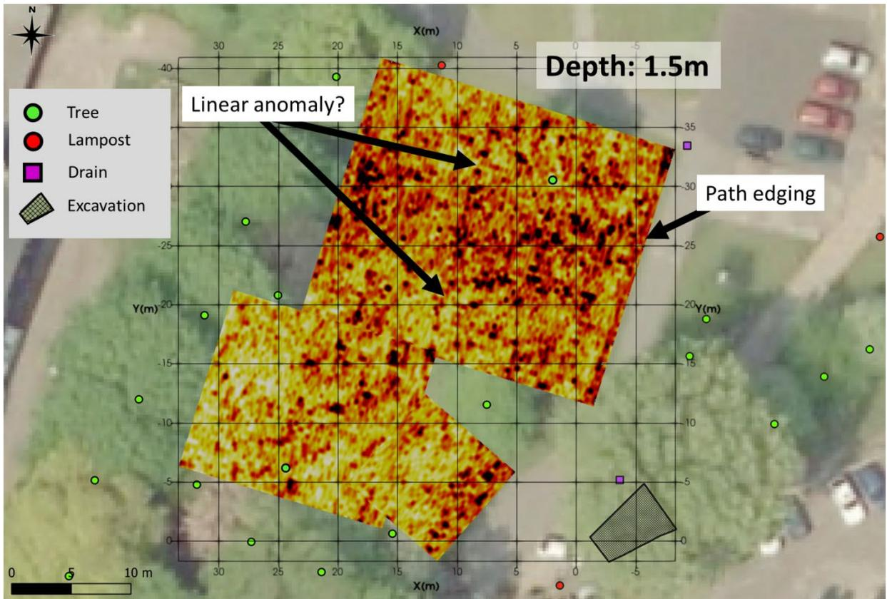
Figure 40: Horizontal slice at 1.5m from 250MHz data.
