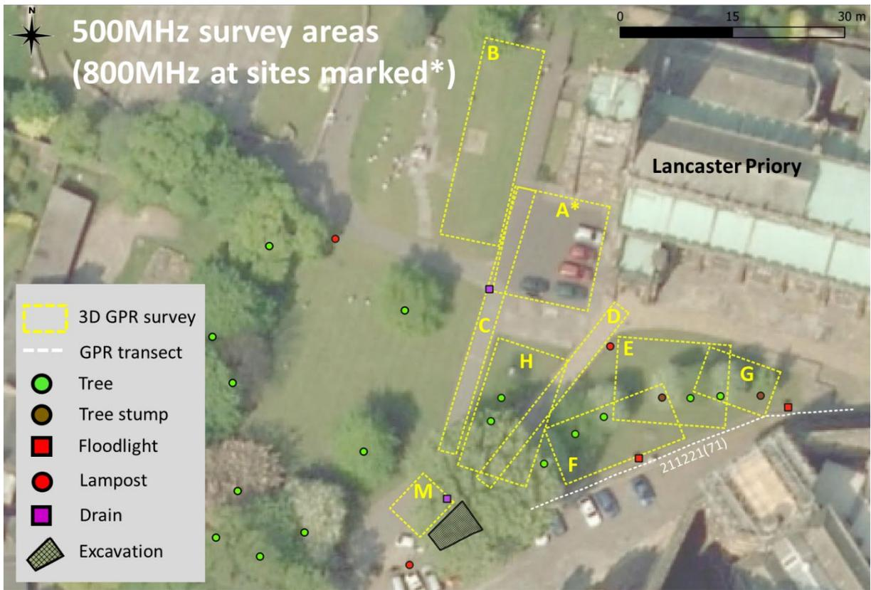
Figure 3: Coverage of 500MHz and 800MHz surveys.
