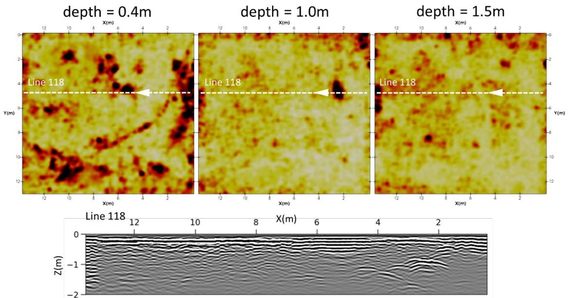
Figure 12: Selected horizontal slices of the 500MHz data, along with an example GPR transect.
