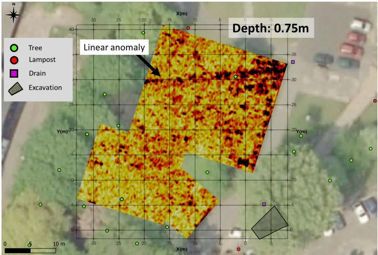
Figure 38: Horizontal slice at 0.75m from 250MHz data.
