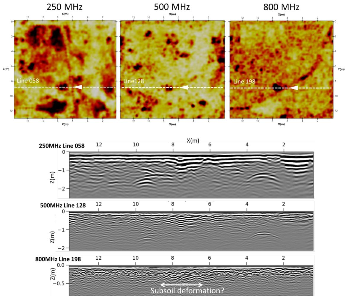
Figure 15: Comparison of 250MHz, 500MHz and 800MHz data. Upper image shows horizontal slice at 0.5m depth. The lower images show an individual trace across the same line for the three antenna frequencies.
