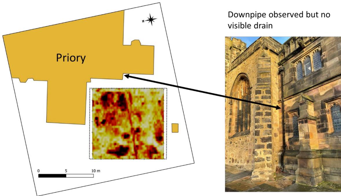
Figure 9: Linear anomaly in Plot A 250MHz horizontal slice at 0.5m depth in relation to existing downpipe.
