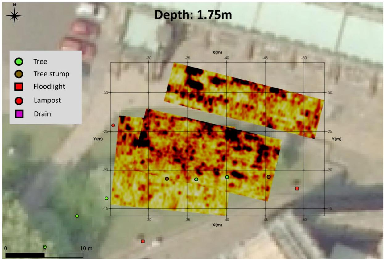
Figure 29: Horizontal slice of 250MHz data from Plots I, Q and R (depth: 1.75m).
