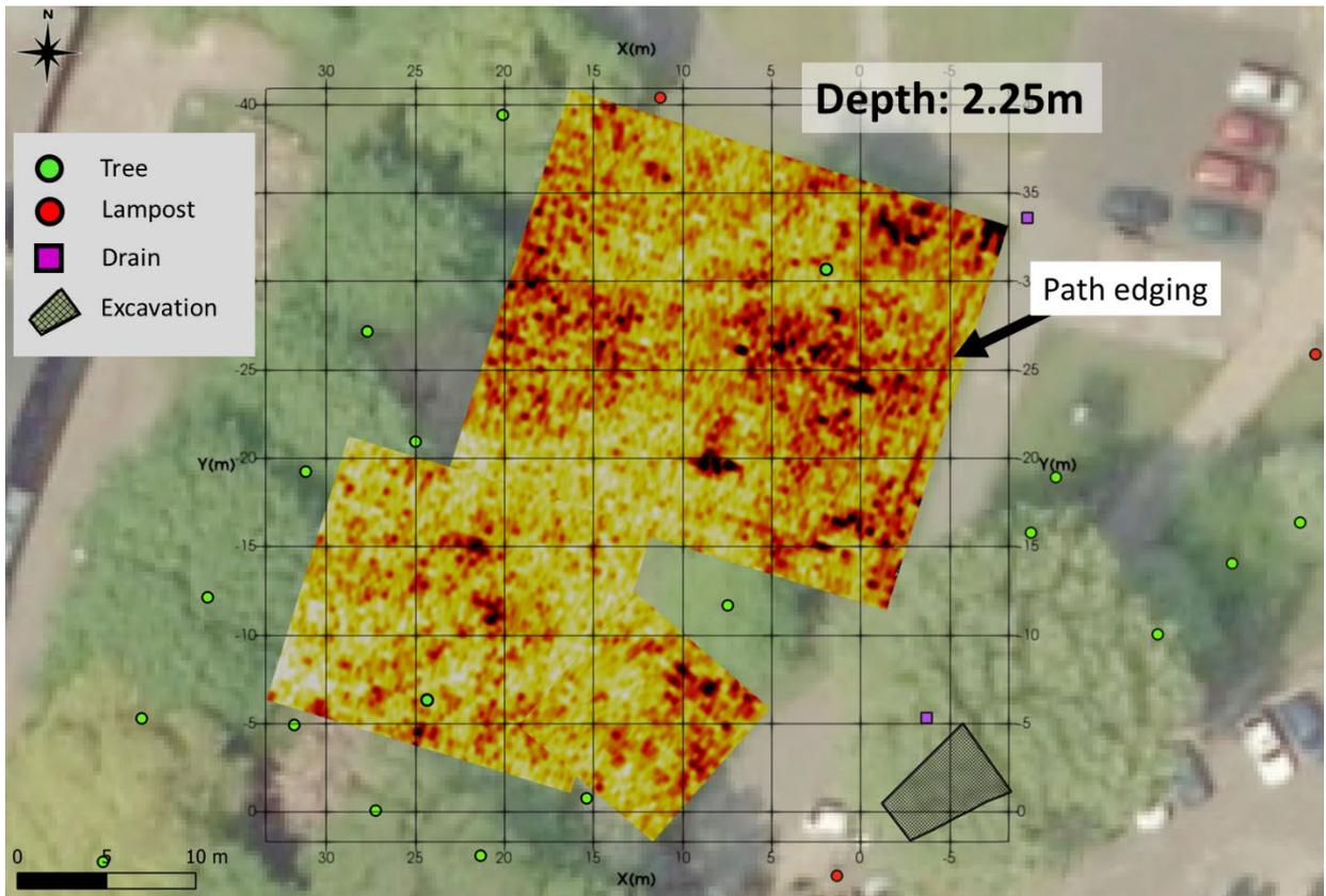
Figure 42: Horizontal slice at 2.25m from 250MHz data.
