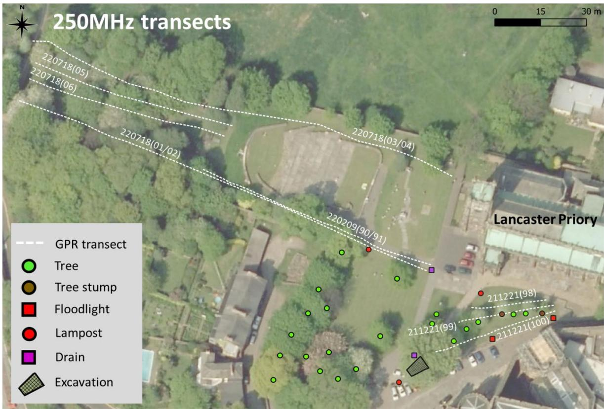
Figure 5: Coverage of 250MHz 2D surveys.
