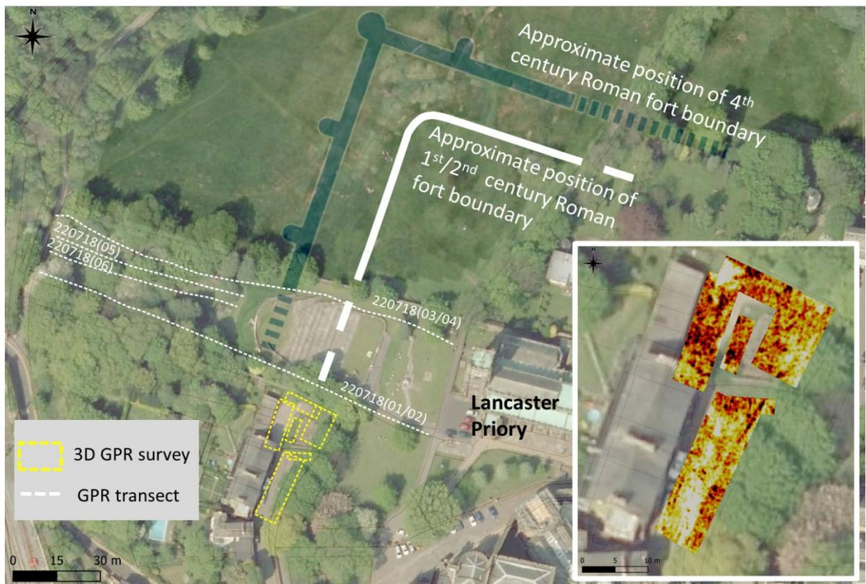
Figure 51: Map showing location of Hillside 500MHz GPR surveys by Binley (2023) in relation to approximate position of Roman Fort boundaries. 250MHz transects shown in Figure 46 are included for reference. The insert image shows Hillside GPR results at a depth of 0.7m below ground level.
