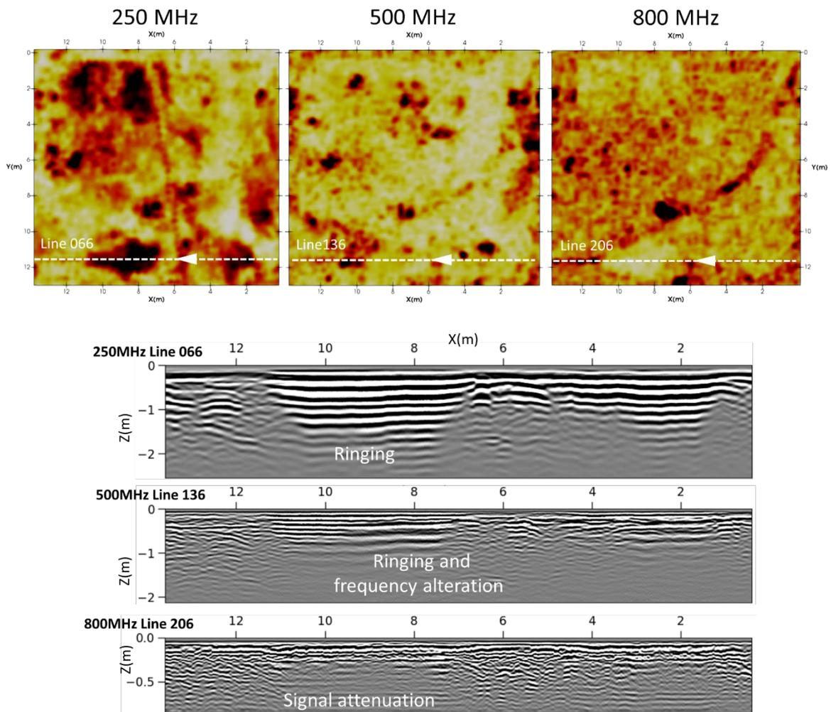
Figure 14: Comparison of 250MHz, 500MHz and 800MHz data. Upper image shows horizontal slice at 0.5m depth. The lower images show an individual trace across the same line for the three antenna frequencies.
