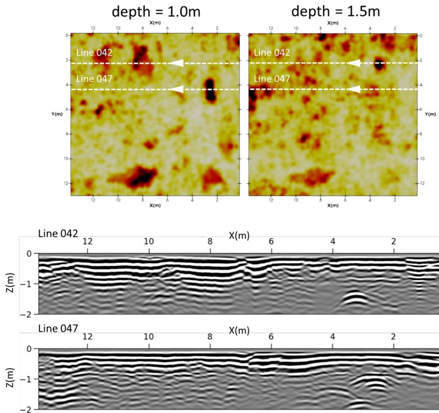
Figure 11: Illustration of localised reflection hyperbolae at depth (250MHz survey for Plot A)
