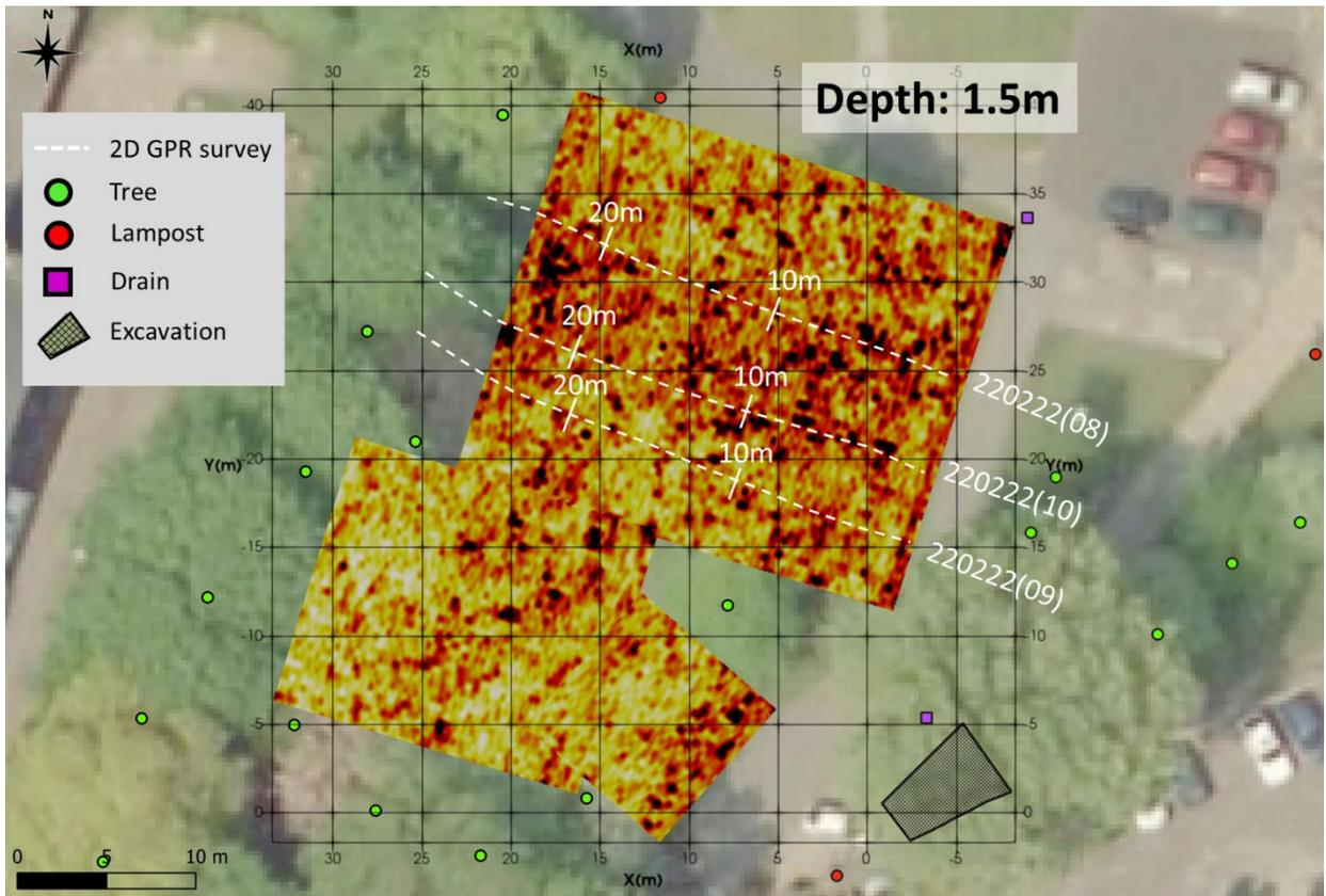
Figure 44: Horizontal slice at 1.5m from 250MHz data and position of three selected 100MHz transects.
