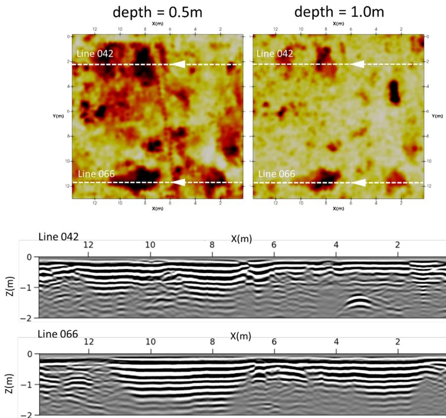
Figure 10: Evidence of 'ringing' behaviour in Plot A 250MHz surveys, illustrated by two individual transects.
