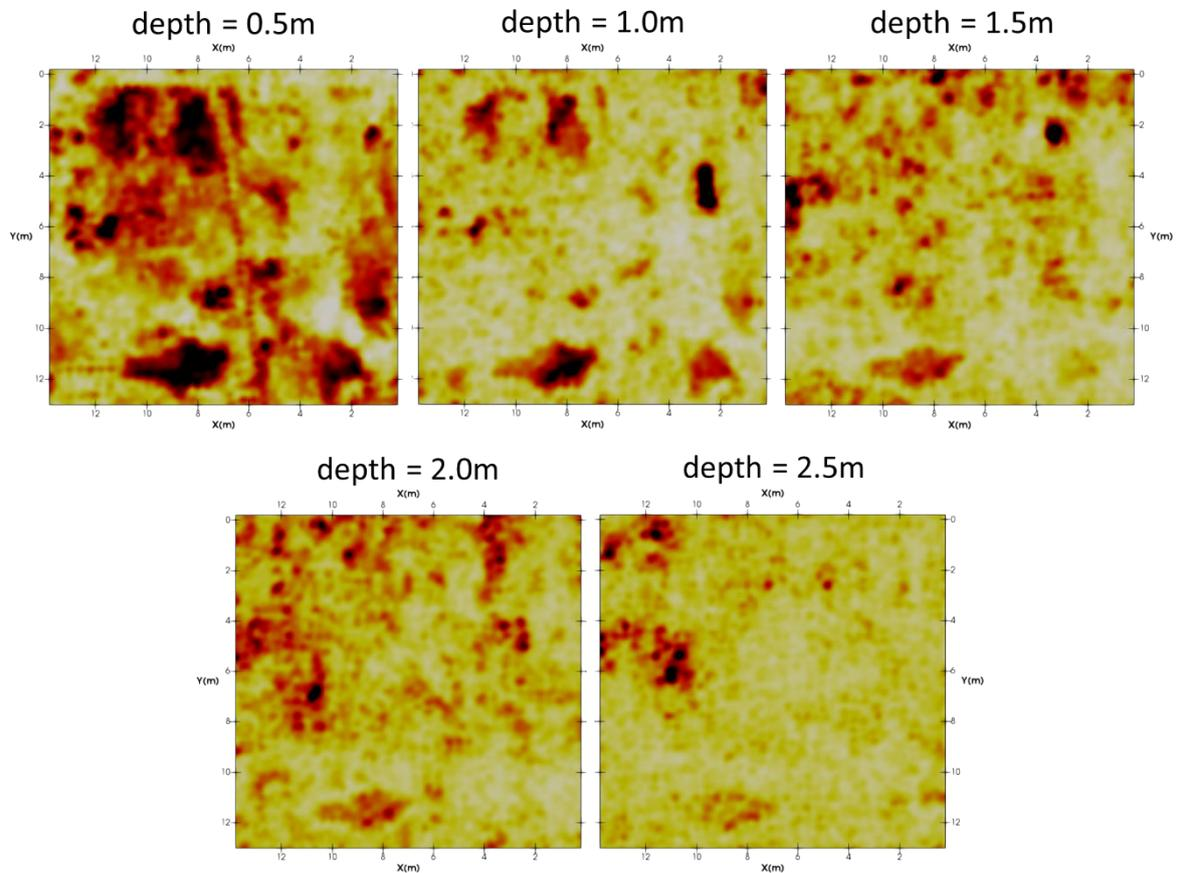
Figure 8: Example horizontal slices of 250MHz data from Plot A. Dark colours indicate reflections.
