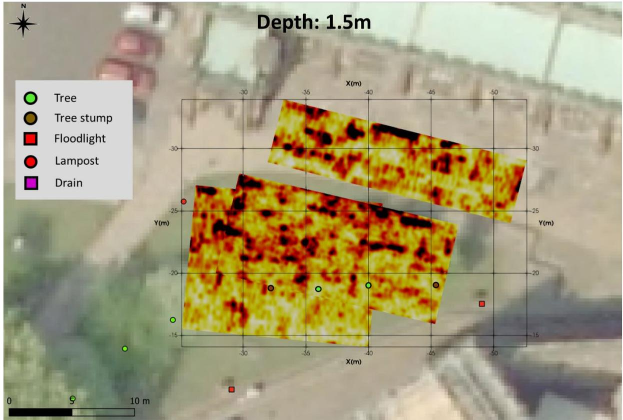
Figure 28: Horizontal slice of 250MHz data from Plots I, Q and R (depth: 1.5m).
