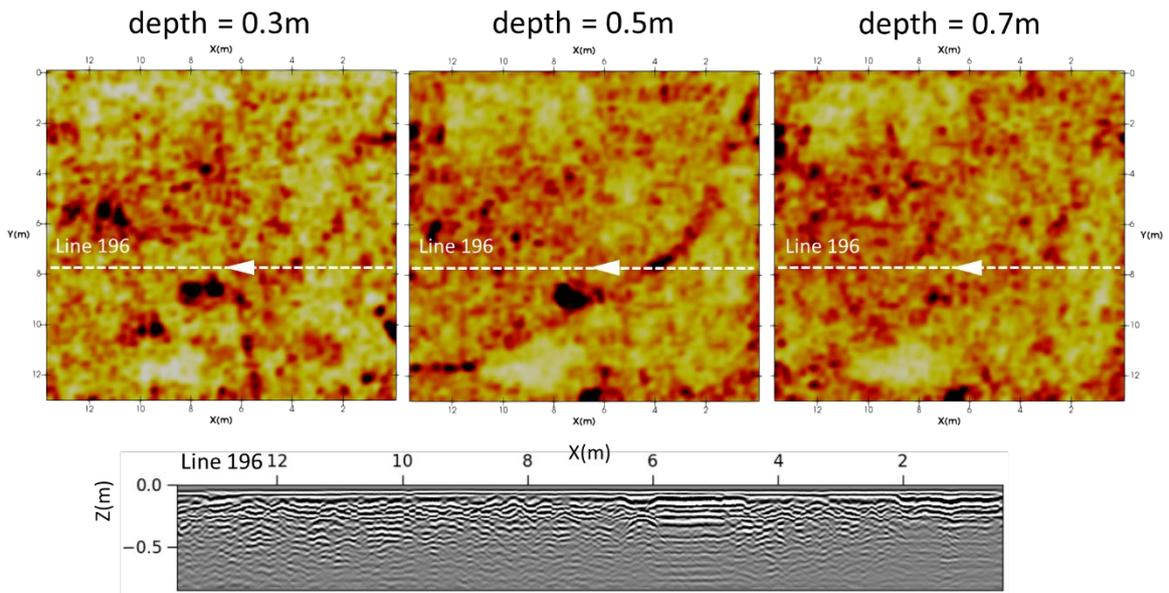
Figure 13: Selected horizontal slices of the 800MHz data, along with an example GPR transect.
