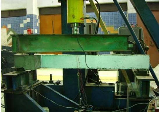
Fig. 3 (b) Details of tested beams and positions of LVDTs
