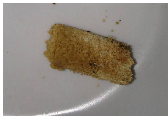
Fig. 9 Sintering of composite catalyst bed after test
