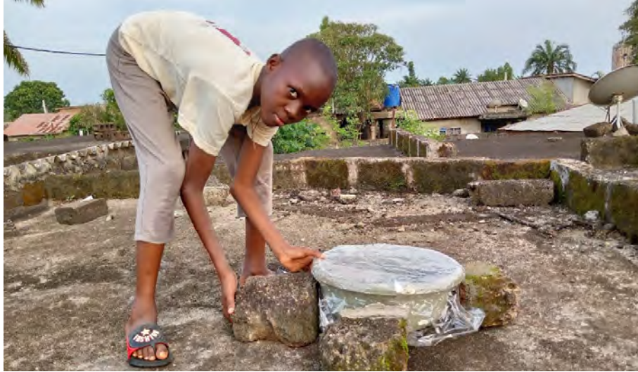
Fig 19: Preparing a trap to collect micrometeorite candidates in Benin (Credit: Pide Aristide Ahanhanzo)
