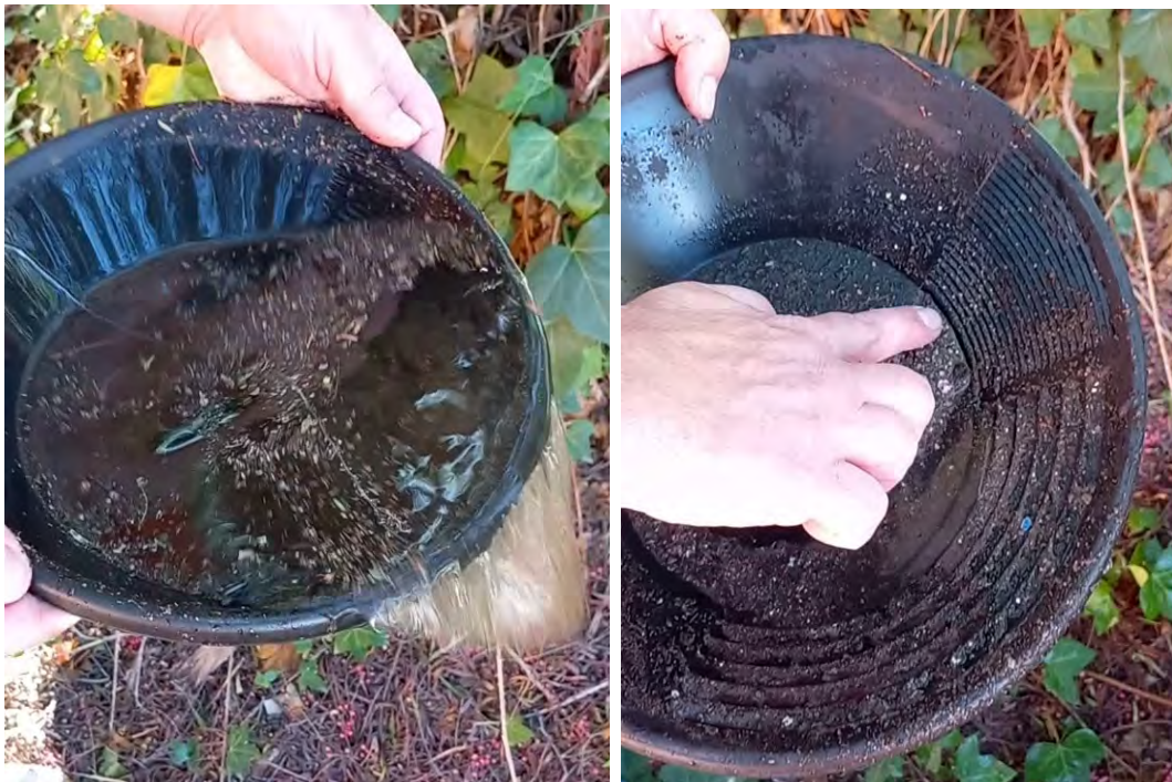
Fig. 63a: Using a gold-washing tray, the water can be decanted and the denser materials left at the bottom of the tray. Fig. 63b: Spherical micrometeorites appear in the background, although they are not ferromagnetic since the effect of magnetism has not been used to detect them (Credit: Stefan Müller-Champrenaud).
