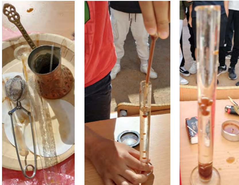
Fig. 4a: In a “casting effect” saucepan, Fig. 4b: Making the drip with a syringe, Fig. 4c: Column of cooling and condensation to form the spheres (Credit: Paula Chis),
