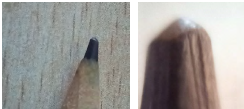
Fig. 10a: Photograph of a pencil lead with a mobile camera, Fig. 10b: Photograph of the lead using a drop of gel on the objective of the mobile or cell phone (Credit: Ricardo Moreno).
