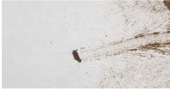
Fig. 8: The magnet, under the sheet of paper, drags the ferromagnetic material (Credit: Beatriz García).
