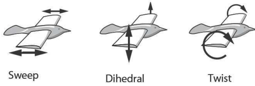
Fig. 1. The flapping motion can be decomposed into three basic motions : sweep, dihedral and twist
