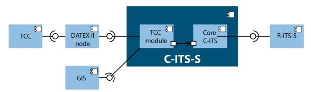
Figure 1. Autostrada del Brennero SpA. Logical scheme of the A22 C-ITS infrastructure
