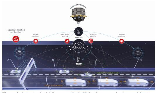
Figure 2. Autostrada del Brennero SpA. Hybrid communication architecture
