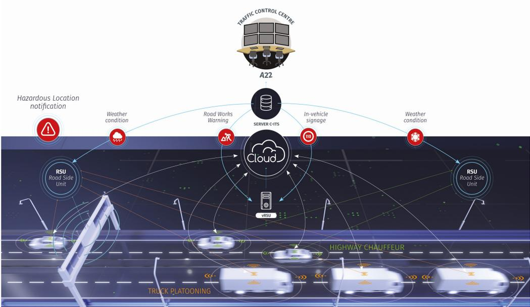
Figure 2. Autostrada del Brennero SpA. Hybrid communication architecture
