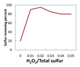
Fig. 1 Sulfur removing percent versus mole fraction changing
