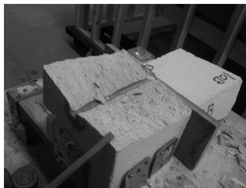
Fig. 3 Total spalling, crushing in front of reinforcement
