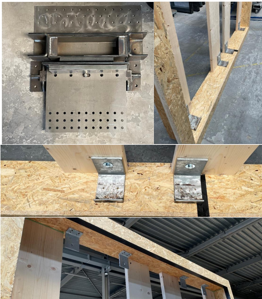
Figure 8: The top and bottom anchors mounted in the test cabinet. Assembled the e-CLT anchor
