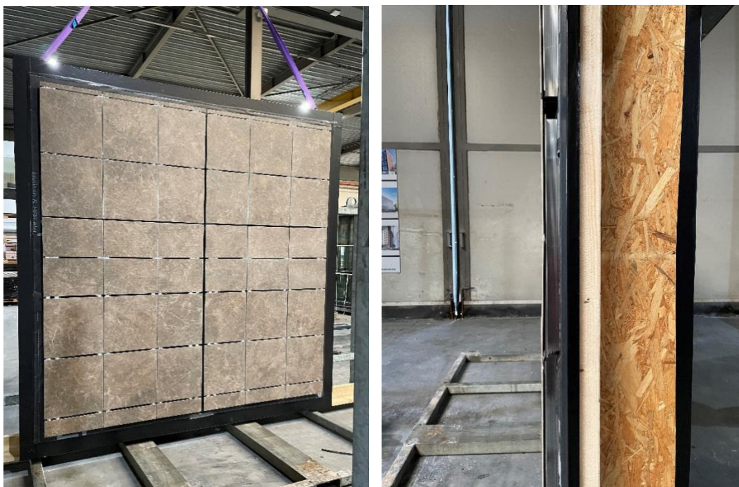
Figure 16: Front view and side view of facade elements in test cabinet
