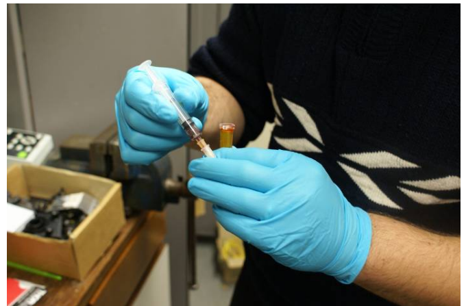
Fig. 11 Applying the fluorescent agent using a syringe
