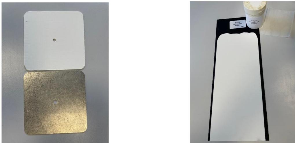
Figure 11. Left Taber aluminium substrate (up coated, down uncoated), right leneta substrate
