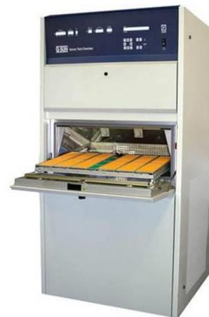
**Figure 14: Q-SUN from Q-LAB, Xenon test chamber**
