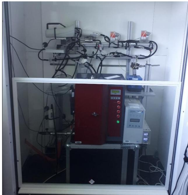
Figure 10 : Overview of the vortex shaker set-up positioned in the variable flow fume hood at CEA.
