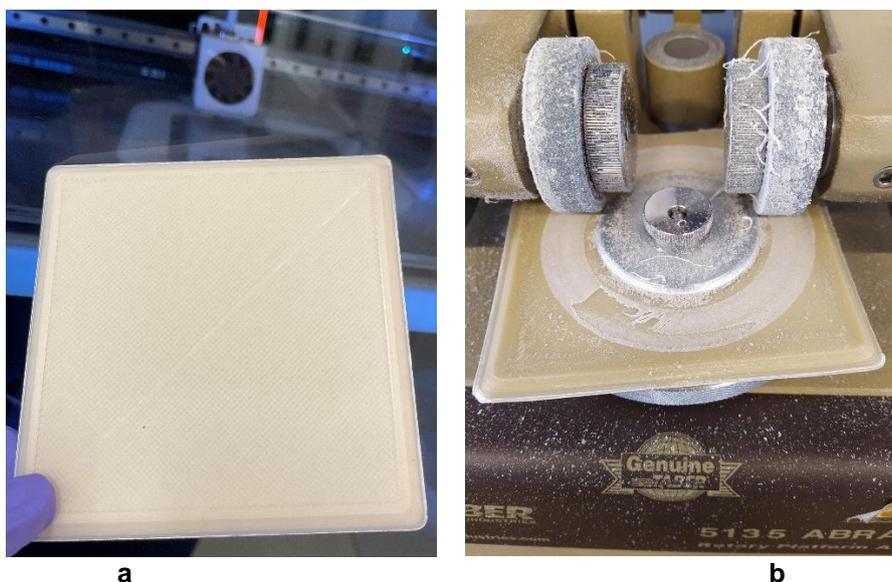
Figure 5. Example of 3D-printed panels before (a) and during Taber abrasion (b).
