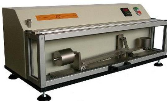
Figure 20. Crockmeter (302, JBA instruments).
