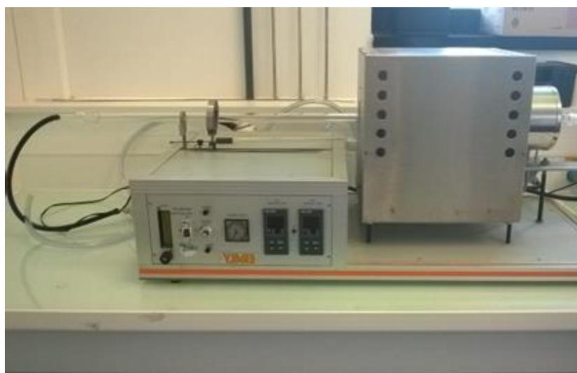
Figure 20. Picture of the tube furnace. From left to right (air flow): introduction tube (room temperature), main furnace (set temperature), auxiliary furnace (180°C).
