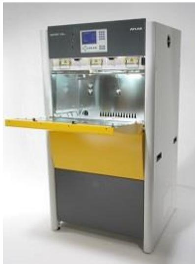
**Figure 12: Suntest XXL, Atlas, Accelerated weathering tester**
