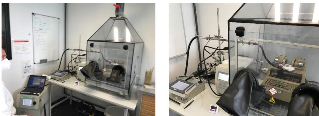
**Figure 18 : Taber abrader placed inside a low background glove box with the associated instrumentation (CEA setup)**
