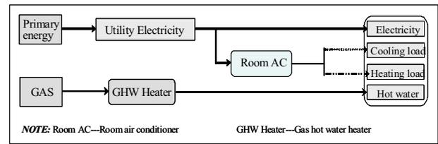
Fig. 2 Energy supply plan of conventional system
