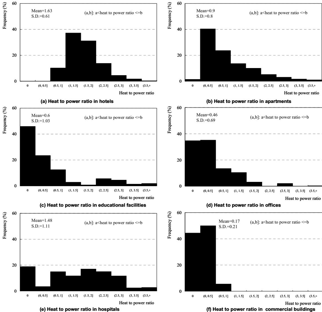
Fig.1: The characteristic of heat to power ratio for various buildings
