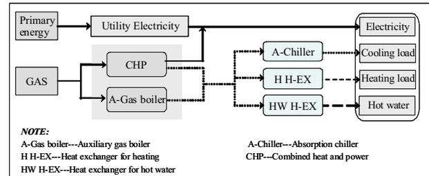
Fig. 3 Energy supply plan of CHP system
