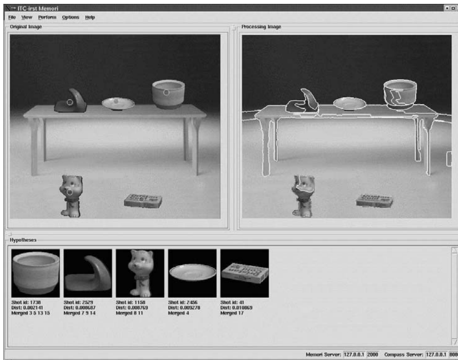
Fig. 20. MEMORI's interface: on left, the input image with the recognized objects highlighted by spots; on right, the segmented image, which it is possible to visualize the region groups corresponding to the recognized objects in; on bottom, the recognized objects are shown along with their identifier number in the input database, the recognition distance computed by considering all the descriptors, and the sequence of merged regions; the scale factor and the orientation angle can be visualized by using the menu options.
