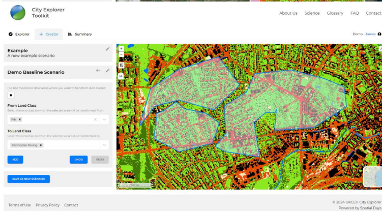
Fig. 2: Screenshots of City Explorer Toolkit. A swipe tool allows easy comparison of layers (top), and users can create their own scenarios to test city plans (bottom).
