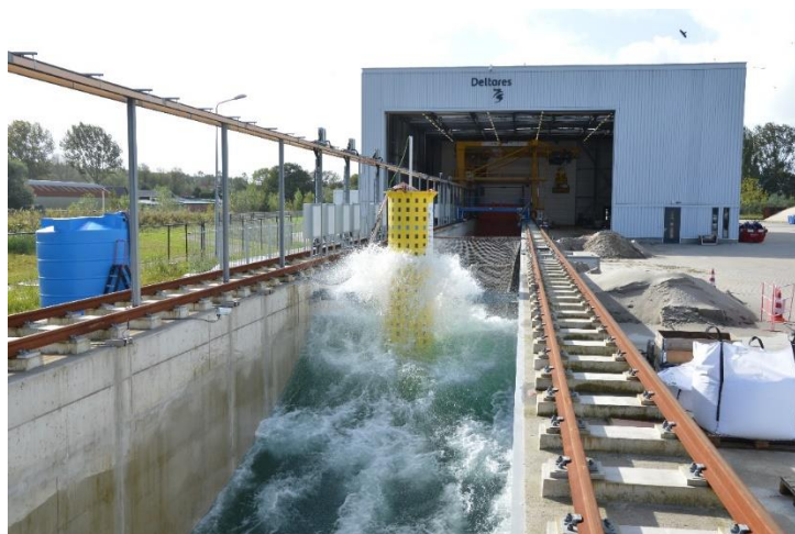
Figure 1 Physical model tests for scour protection performance in Deltares' Delta Flume.
