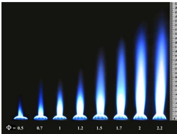
Fig. 9 LPG with 50% Hydrogen IDFs, Re=3000
