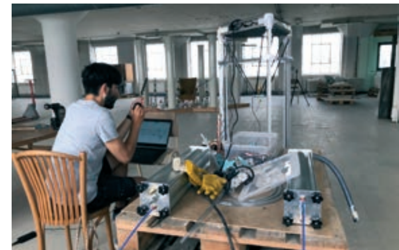
A new dual extrusion 3D printer for clay was built by José Hernández Vargas to be able to print two different coloured batches of clay in alternating layers, Ifö Center in Bromölla, 2020. Photo: Helena Westerlind
