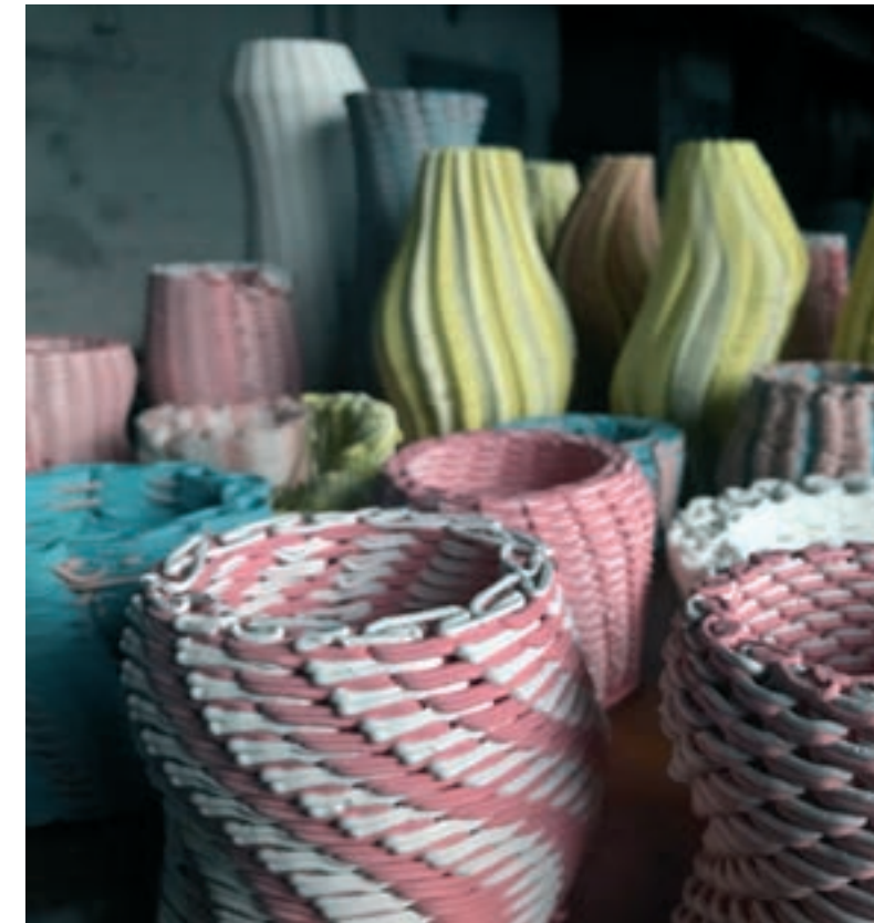
Printed prototypes based on different combinations of "stitches" and colours, Ifö Center in Bromölla, 2020. Photo: Helena Westerlind
