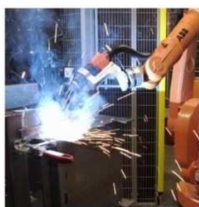
(b) welding in operations
