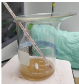
Figure 3. Set up for Fenton oxidation: a 600 mL beaker containing 20 mL Fe(II) solution and 20 mL H 2 O 2 , a magnetic stir bar, thermometer, and an evaporating dish as a cover. The hotplate is set to 75 °C and the stir plate to 190 rpm.
