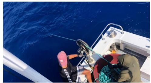
Figure 104. The umbilical of the Azor drift-cam showing a very wide angle on the winch. This is indicative of strong drift and/or strong bottom currents, 22 August 2023.
