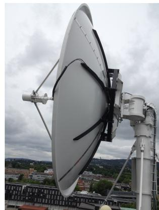
Figure 4: The X/L band antenna in Oslo.
