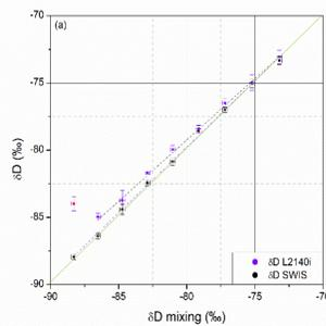
Comparison between SWIS and Picarro L2140i instruments for the analysis of nine samples with respect to the expected values calculated from the volumetric mixing of the standard waters. Linear correlations were obtained with slopes of  $0.981 \pm 0.014$  (SWIS) and  $0.912 \pm 0.014$  (L2140i) for the  $\delta D$  (a), and  $0.995 \pm 0.046$  (SWIS) and  $0.909 \pm 0.036$  (L2140i) for the  $\delta^{18}O$  (b).
