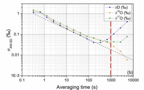
Evaluating long-term stability of the instrument using the Allan standard deviation statistical analysis on 5 hours continuous measurements of milliQ water at 20°C.
