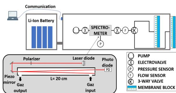
Operating diagram of SWIS. For Borehole applications the Li-Ion battery is integrated in the same Ti-housing of the instrument.
