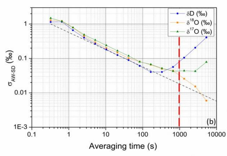
Evaluating long-term stability of the instrument using the Allan standard deviation statistical analysis on 5 hours continuous measurements of miliQ water at 20°C.
