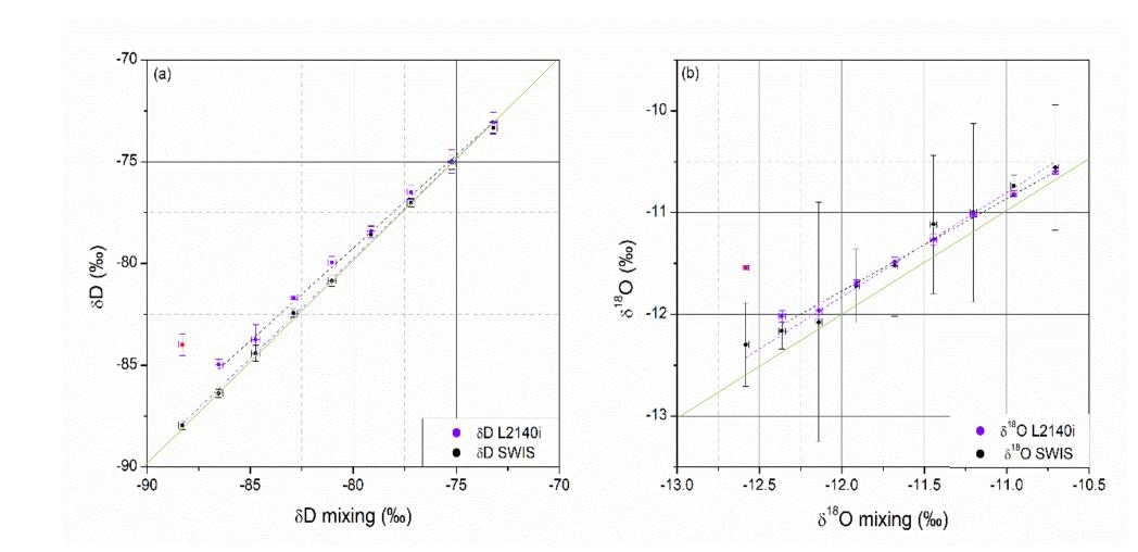
**Comparison between SWIS and Picarro L2140i instruments** for the analysis of nine samples with respect to the expected values calculated from the volumetric mixing of the standard waters. Linear correlations were obtained with slopes of  $0.981 \pm 0.014$  (SWIS) and  $0.912 \pm 0.014$  (L2140i) for the  $\delta D$  (a), and  $0.995 \pm 0.046$ (SWIS) and 0.909  $\pm$  0.036 (L2140i) for the  $\delta$  <sup>18</sup>0 (b).
