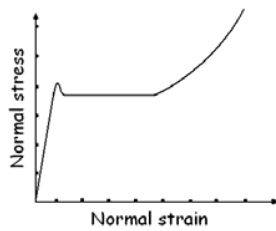
Fig1. Foam behavior in uniaxial compression
