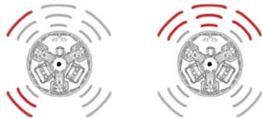
Fig. 8. Two examples of a metaphor for an intuitive representation of distance values. The visualization is in style of a parking distance control of a car. The center of each example shows a top view of the robot.
