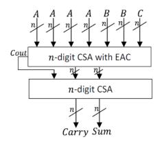
Fig. 5 Converter for modulus  $r^n - 2$  where r = 7,9,11
