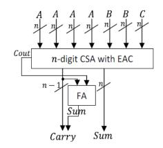
Fig. 6 Converter for modulus  $r^n - 2$  where  $r \ge 13$
