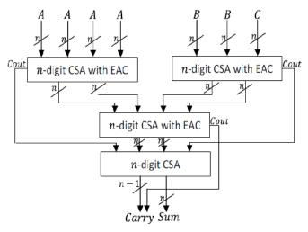
Fig. 3 Converter for modulus  $3^n - 2$  where  $n \ge 4$
