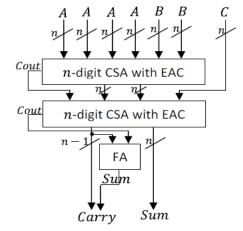
Fig. 4 Converter for modulus  $5^n - 2$
