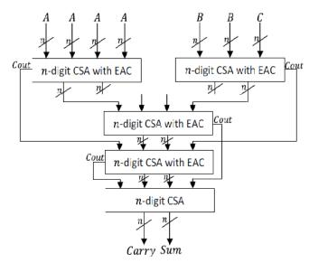
Fig. 2 Converter for modulus  $3^n - 2$  where n = 2, 3
