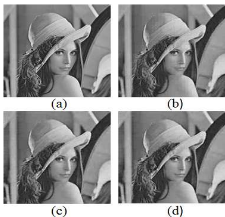
Fig. 2 (a) the 256-grayscale standard image "Lenna" with 256 \times 256 pixels, (b) the JPEG-compressed image converted by the lossy JPEG image compression ( q=2 , MSE=83.26 ), (c) the grayscale image obtained by the MPM estimate when q=2 , J=0.23 , T_m=1 and h=1.0 ( MSE=91.87 ), (d) the grayscale image obtained by the MPM estimate when q=2 , J=0.31 , T_m=1 and h=1.0 ( MSE=77.85 )
