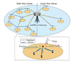
Figure 7: mmWave meshed network overlaid on a LTE macro cell.
