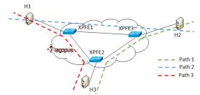
Figure 4: Test scenario and instantiated paths for EMMA experiments on XPFEs domain
