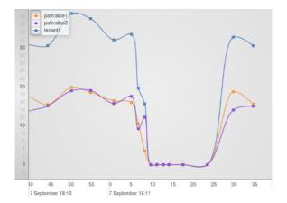
Figure 3: Screenshot of power consumption monitoring per service and per tenant over time
