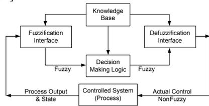
Fig. 3 Basic configuration of fuzzy logic controller (FLC)
