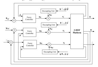
Fig. 2 Multivariable fuzzy control for the 3-DOF platform
