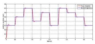
Fig. 7 Tracking performance using TS fuzzy controller with adaptive decoupling scheme
