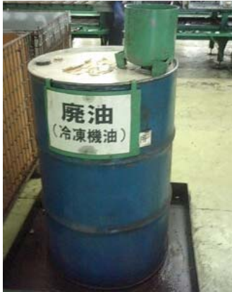
Fig. 8 Waste Oil Divided from Waste Home Appliances
