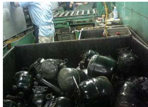
Fig. 6 Compressors Divided from Waste Home Appliances
