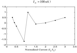
Fig. 4 Errors between the simulated and the theoretical results (@ $I_{in} = 100 nA$ )
