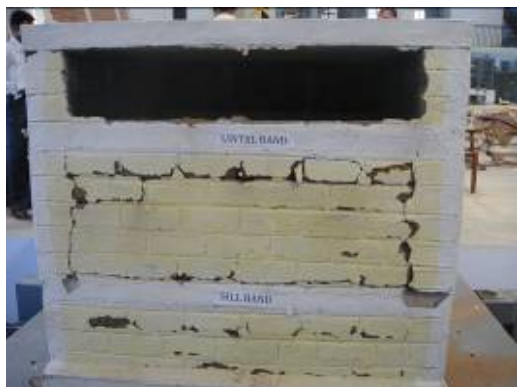
Fig. 14 Final Collapse – Model S2
