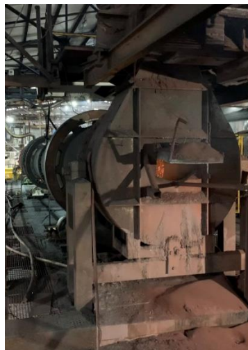
Figure 2 High temperature cylindrical oven at ILPEA
