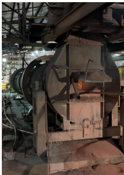
Figure 2. High temperature cylindrical oven at ILPEA
