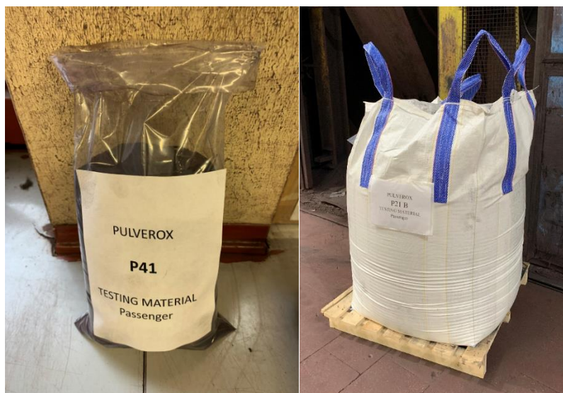
Figure 9. Improved Sr-ferrite materials produced by ILPEA in the framework of PASSENGER, achieving a production of 4 tones already at this stage (M24) in the project.
