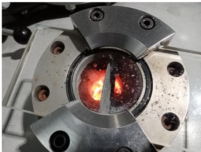
Figure 2: Production of MnAlC alloy by LCM
