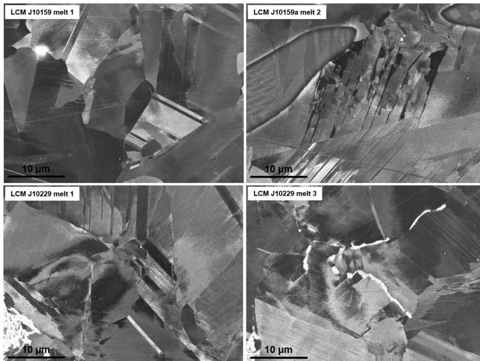
Figure 6 - High-resolution electron channelling contrast (ECC) images of samples which were prepared by LCM.
