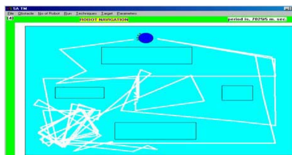
Fig. 7. The path traced by 4 mobile robots controlled using the RBF
